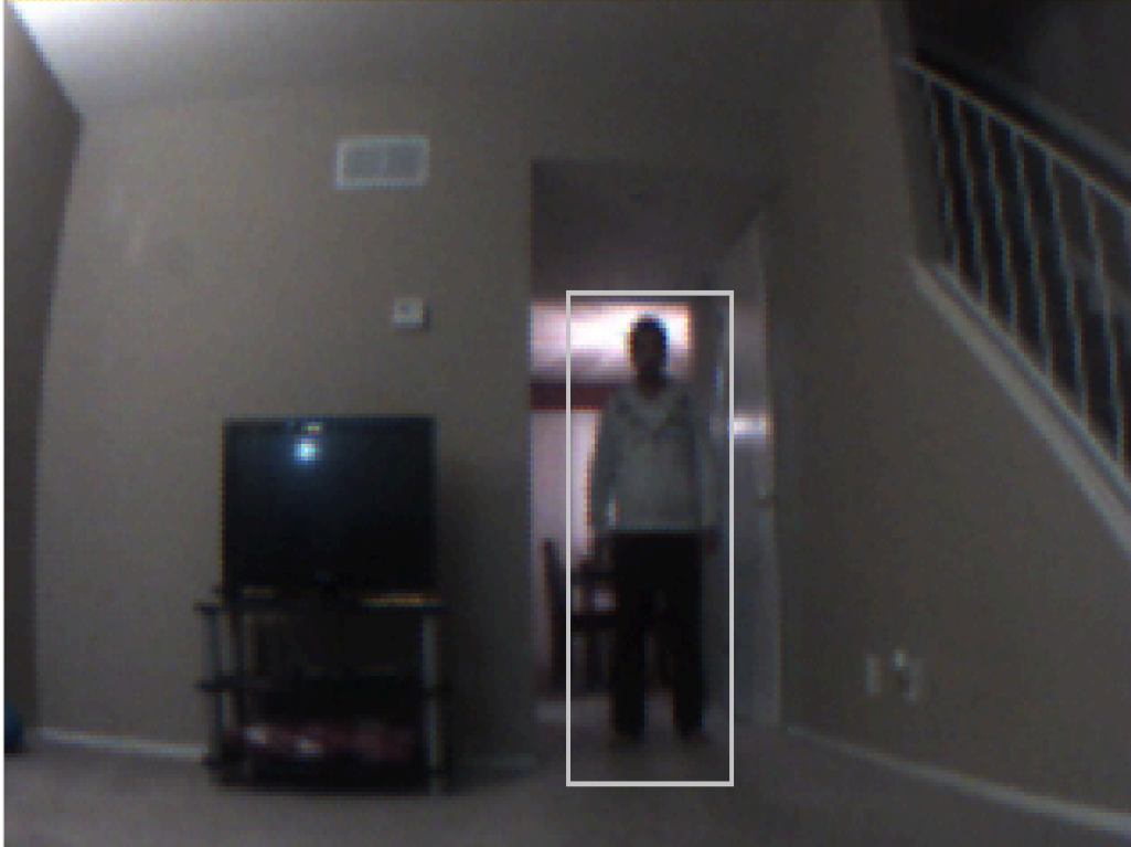
Figure 47 – Smart surveillant detects a person’s presence motion detected as intrusion (The box in second image is manually done; frame differencing does not box the objects)
